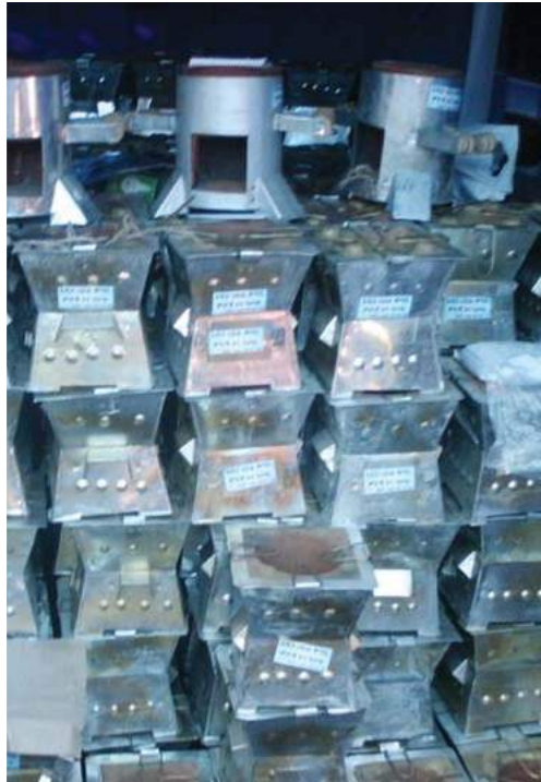
Local Entrepreneurs in Addis Abeba producing and storing two types of improved cookstoves. Each significantly reduces biomass fuel consumption and carbon emissions per cooked meal Photo credit: Getu Shikur
