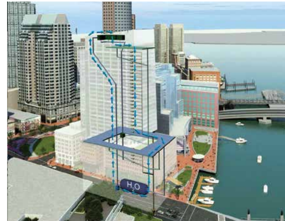
By making use of harvested rainwater, Boston Properties' Atlantic Wharf building is designed to use 15% less water in building HVAC systems compared to a typical building. This illustration shows the flow of harvested water through the building.
